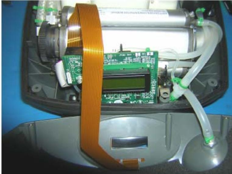
**Figure 17: Membrane Panel Ribbon Cable Installation.**
