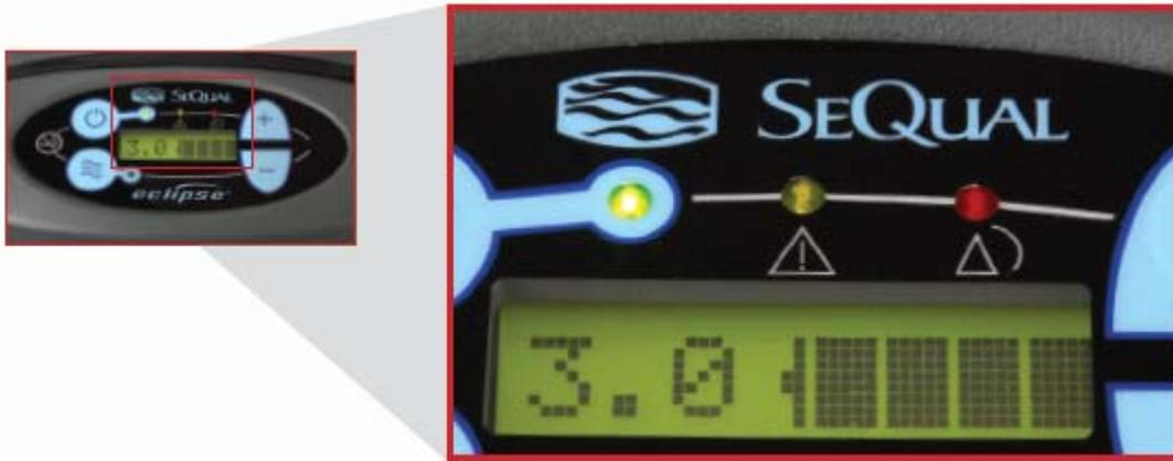
**Figure 8: Power Cartridge Status Gauge**
