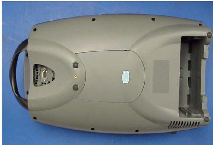
**Figure 12: Removing screws to open the Front Cover**
