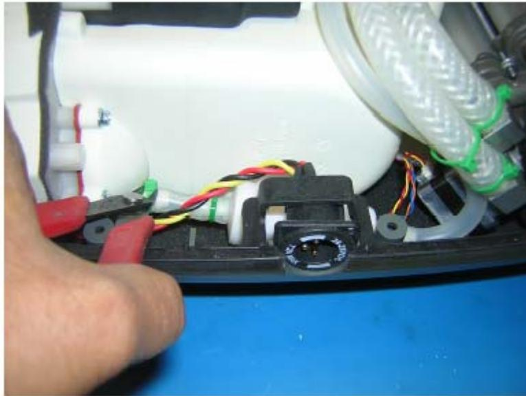
**Figure 23: Removing the Compressor Intake Filter.**
