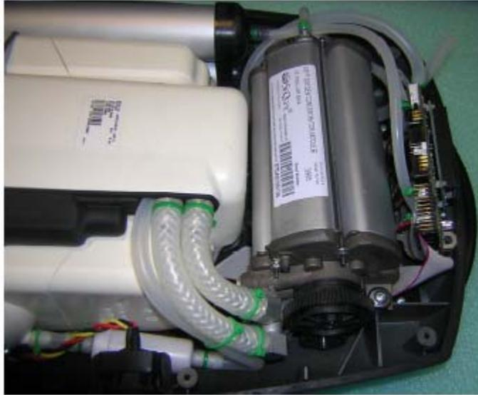
**Figure 24: Installing the Compressor Intake Filter.**
