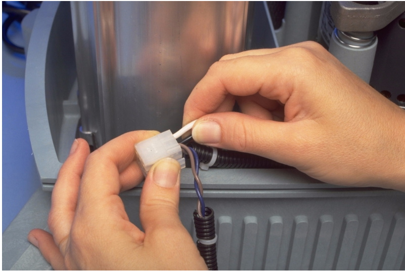
FIGURE AY: REMOVING THE POWER CORD WIRES FROM THE MAIN POWER WIRING HARNESS
