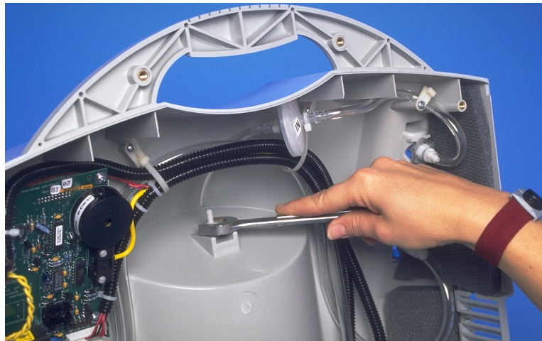
FIGURE L: REMOVING THE JAM NUT
