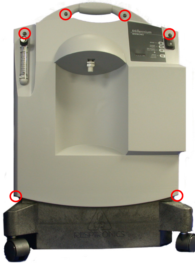
FIGURE E: FRONT CABINET SCREW LOCATION
