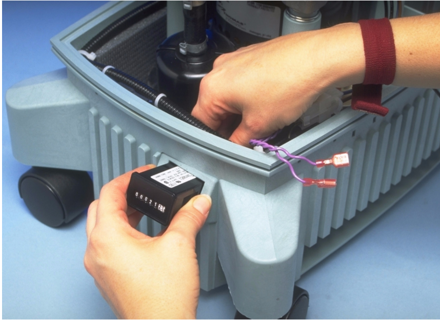
FIGURE AR: REMOVING THE HOUR METER
