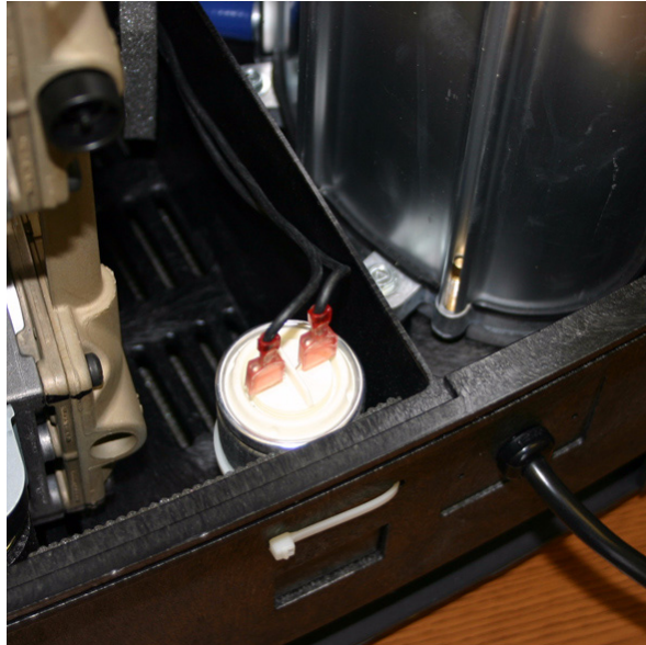
FIGURE AE: CAPACITOR LOCATION
