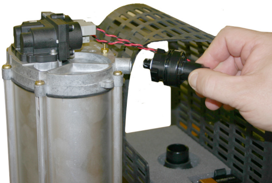
FIGURE AK: REMOVAL OF THE PRESSURE REGULATOR
