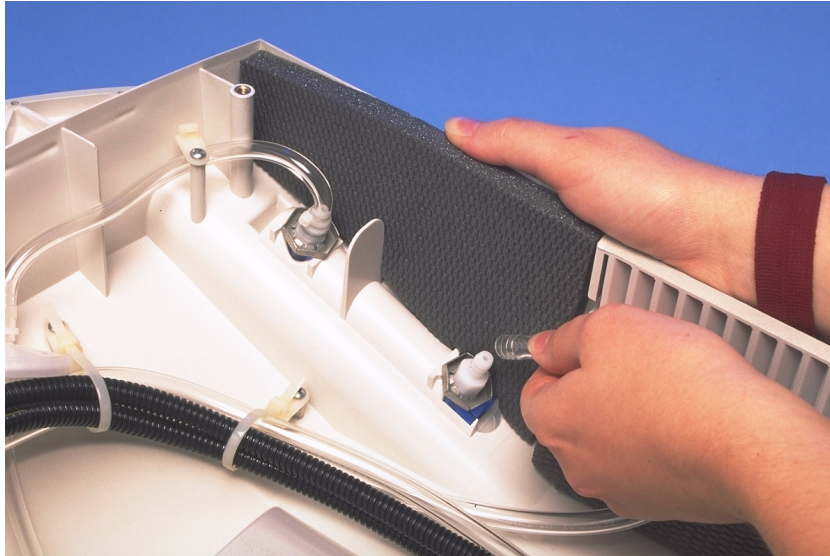
FIGURE H: REMOVAL OF PRESSURE TUBING FROM FLOW METER
