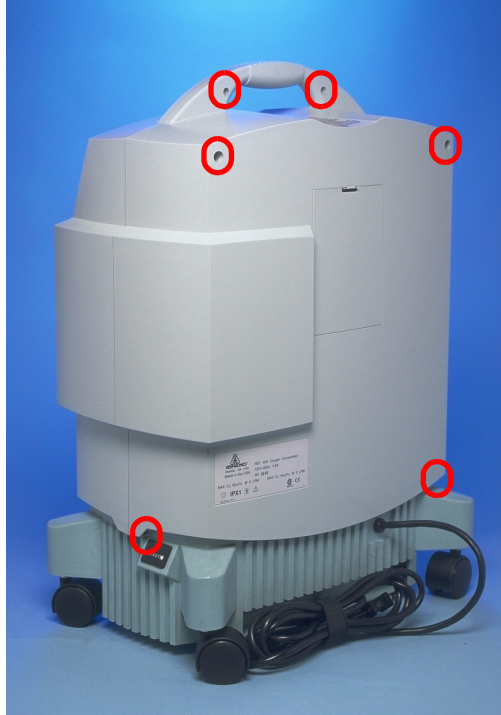
FIGURE E: REAR CABINET SCREW LOCATIONS
