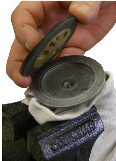
FIGURE AD: REPLACE PISTON CUP
