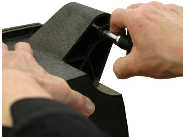
FIGURE B: REMOVING THE CASTER
