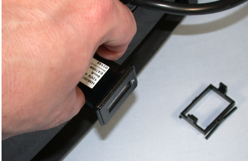
FIGURE AK: REMOVAL OF HOUR METER
