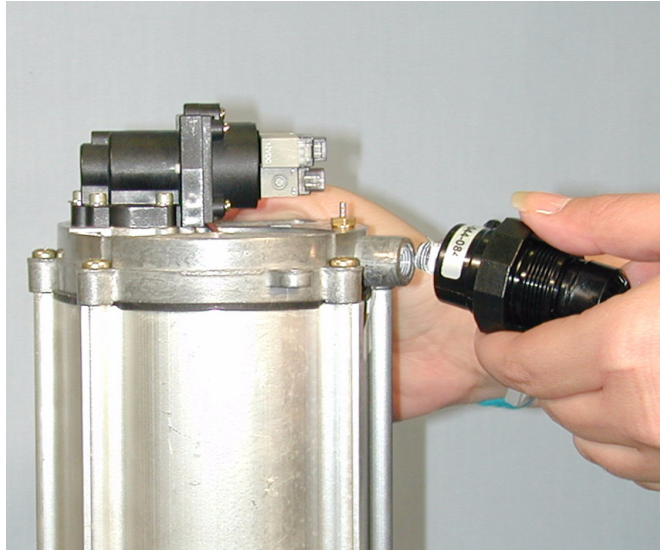
FIGURE AM: REMOVAL OF THE PRESSURE REGULATOR
