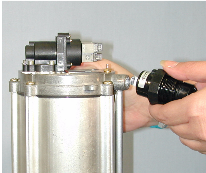
FIGURE AU: REMOVING THE PRESSURE REGULATOR
