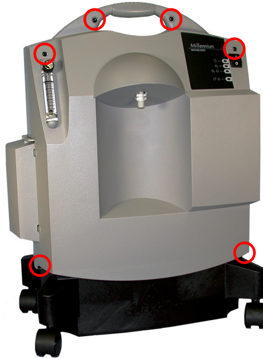
FIGURE E: SCREW LOCATIONS
