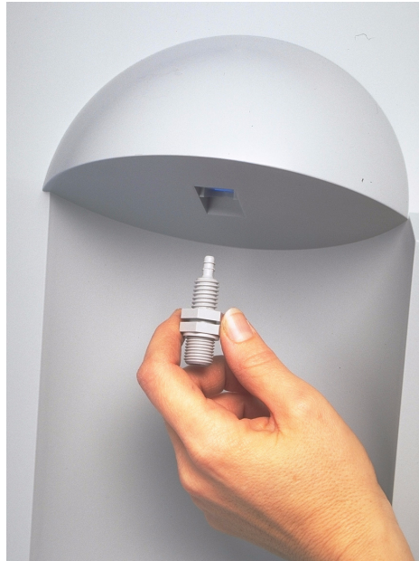
FIGURE M: REMOVING THE DISS FITTING
