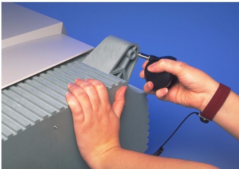
FIGURE B: CASTER REMOVAL
