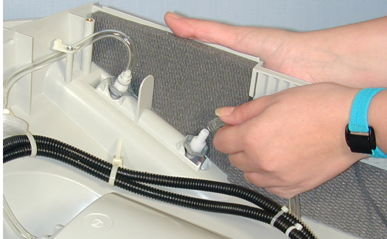
FIGURE G: REMOVE THE PRESSURE TUBING FROM THE FLOW METER
