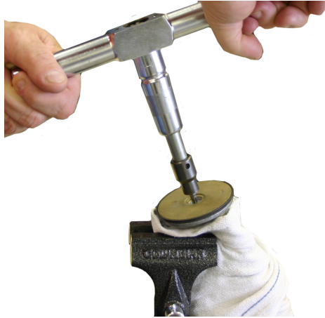
FIGURE AC: SCREW REMOVAL
