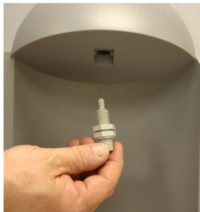
FIGURE I: REMOVING THE DISS FITTING
