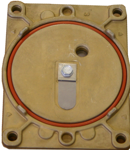
FIGURE W: CYLINDER SIDE OF VALVE PLATE
