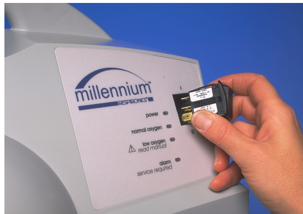
FIGURE P: REMOVING THE POWER SWITCH FROM THE FRONT CABINET ASSEMBLY
