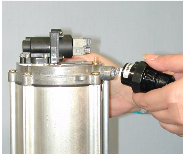
FIGURE AM: REMOVAL OF THE PRESSURE REGULATOR
