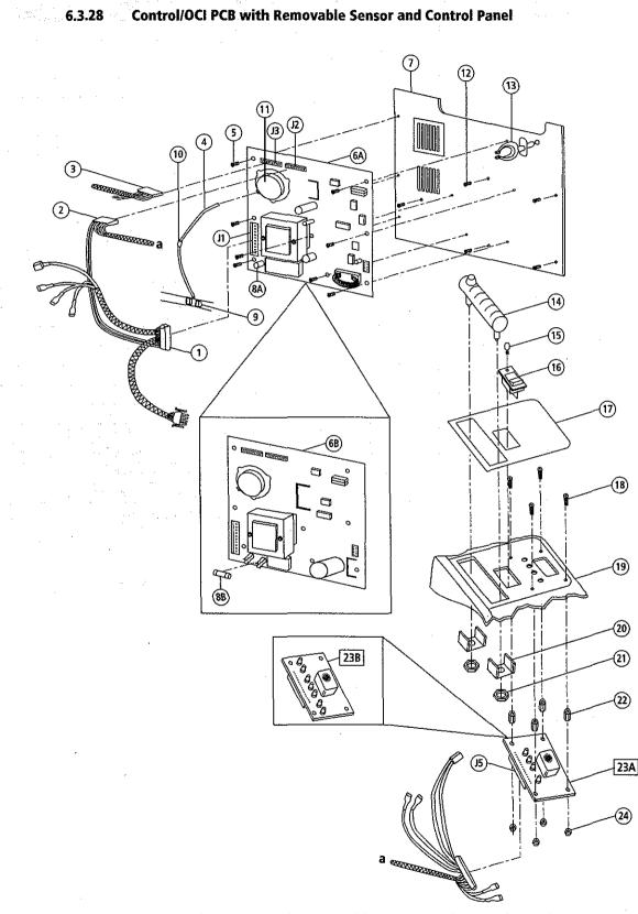
Figure 6-26: Control/OCI PCB with Removable Sensor and Control Panel
