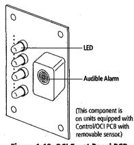
Figure 1-19: OCI Front Panel PCB
