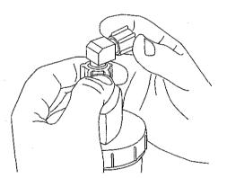
Figure 7-6: Humidifier Adapter Attachment
