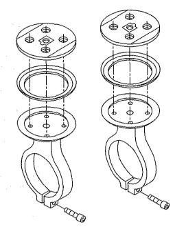
Figure 5-1: Retaining Plates
