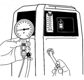
Figure 3-5: Outlet Pressure Testing
