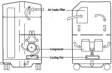
Figure 7-4: Cooling Air Flow
