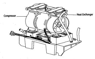
Figure 1-5: Compressor Platform, Front View
