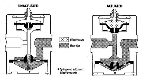
**Figure 1-9: Pilot Valve Operation**
