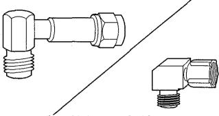
Figure 7-5: Oxygen Outlet Adapters
