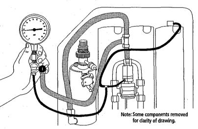
Figure 3-2: Pneumatic Test Kit Connection
