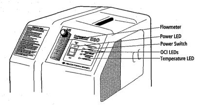
Figure 1-16: OCI Indicator LEDs
