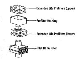
Figure 1-3: Compressor Inlet Extended Life Prefilters
