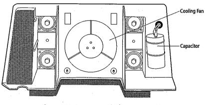
Figure 1-21: Compressor Platform, Bottom View
