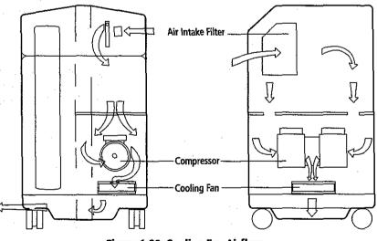
Figure 1-20: Cooling Fan Airflow
