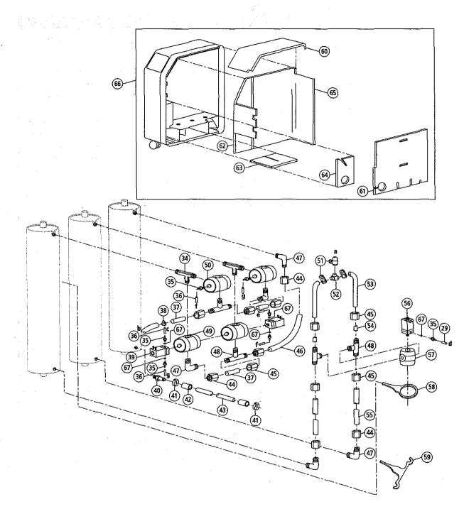
Figure 6-3b: Left Cabinet Interior with Non-O-Ring Fittings
