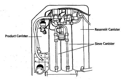
Figure 1-6: Reservoir, Sieve, and Product Canisters
