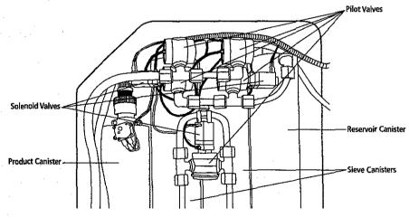
Figure 1-8: Solenoid and Pilot Valves
