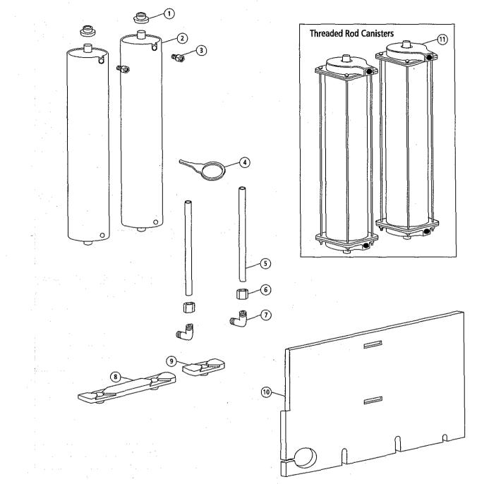
Figure 6-5: Retrofit Sieve Bed Assembly
