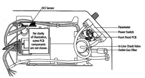
Figure 1-14: Right Cabinet Interior (Control/OCI PCB with Removable Sensor)
