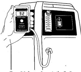
Figure 7-3: Oxygen Concentration Testing
