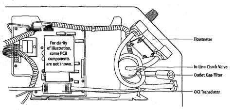
Figure 1-13: Right Cabinet Interior (Control/OCI Combo PCB)
