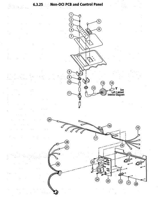
Figure 6-23: Non-OCI PCB and Control Panel
