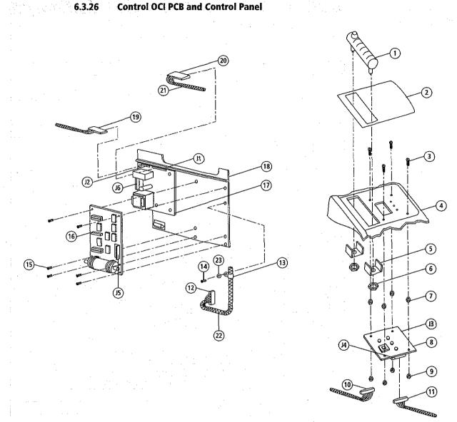
Figure 6-24: Control OCI PCB and Control Panel
