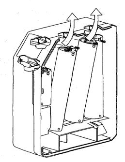
Figure 5-2: Sieve Canister Removal
