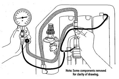
Figure 3-4: Pressure Switch Testing
