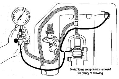
Figure 3-3: Pressure Test, Reservoir Canister
