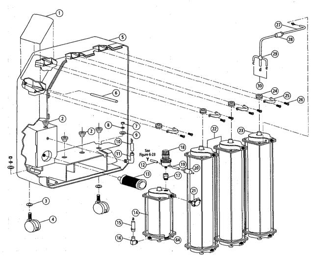
Figure 6-2a: Left Cabinet Interior with Threaded Rod Sieve Beds
