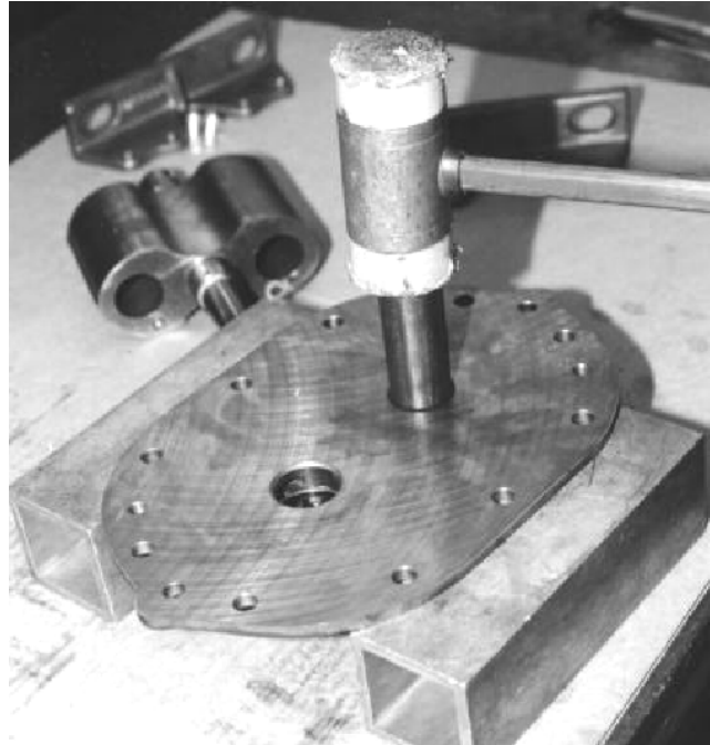
Figure 11. Tapping Bearings Out of End Plates.
