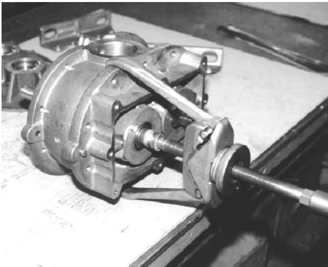
Figure 10. Driving Rotors Out Using Jaw Puller.
