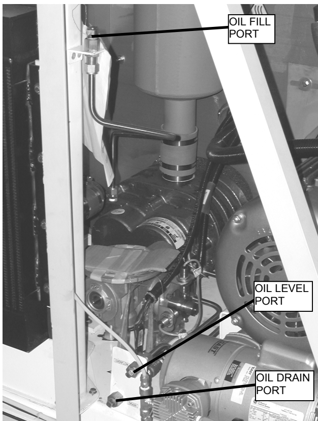
Figure 18. Blower Gear Case Oil Ports.
