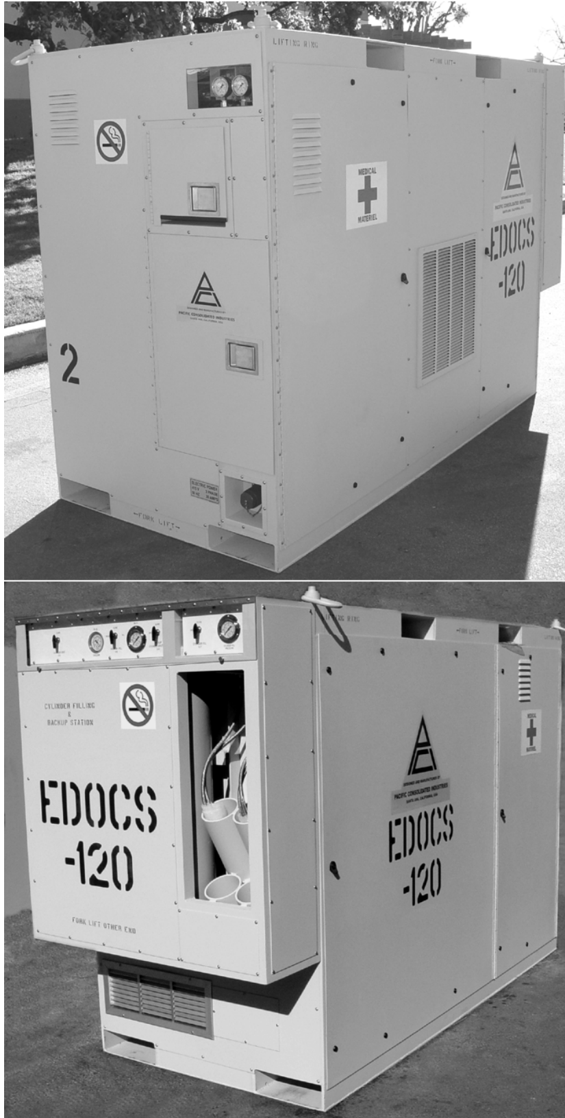
Figure 1. Expeditionary Deployable Oxygen Concentration System (EDOCS-120).
